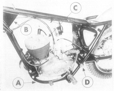
New J-Be-Sachs 200cc "Sport" and "Scrambler" both have the following features: A—Heavyduty, full engine width cradle frame for maximum crankcase protection, B-Duplex gusset for additional frame strength where most needed, C-Fourteen horsepower Sachs engine, D-Heavythe oversize brakes. Wheels are heavy-duty duty swinging arm spindle with handy grease nipple.
